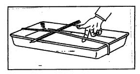
Placing the bridge at the quarter point will give the next octave. Also try to produce the familiar do-misol-do of the major chord by using the "open" string then placing the bridge at distances 1/5, 1/3 and 1/2 from the left end, each time plucking the right hand portion of the string. Another fact you can check is that tightening a string raises its pitch.
